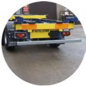
Galvanised Rear Pull Out Crash Bar And Bolt On Light Brackets
