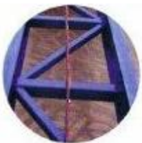
Main Chassis Strengthened With Diagonal Style Box Section Braces
